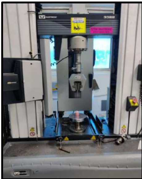
Fig 28 : Universal testing machine
