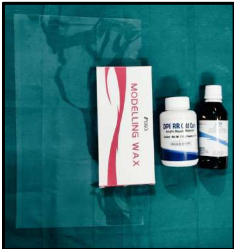
Fig 6 : Materials for mold preparation 6 (a). Polyvinyl chloride sheet 6 (b). Modelling wax 6 (c). Self Cure Powder 6 (d). Self cure liquid
