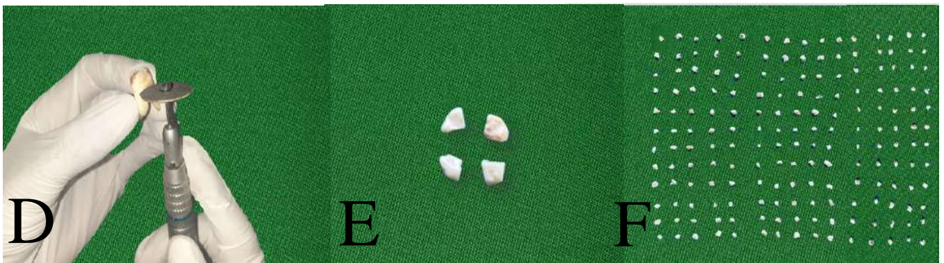
Fig.3D: Sectioning of the tooth.
