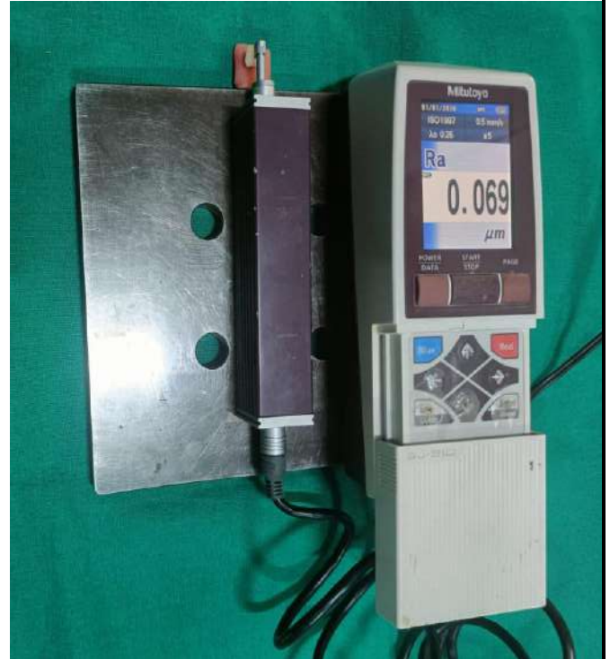
Fig 18- Surface abrasiveness test of sample using profilometer
