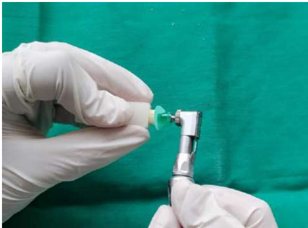
Fig 15- Finishing and polishing of the sample
