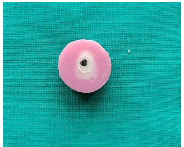
Fig 16- Sample mounted on acrylic for testing
