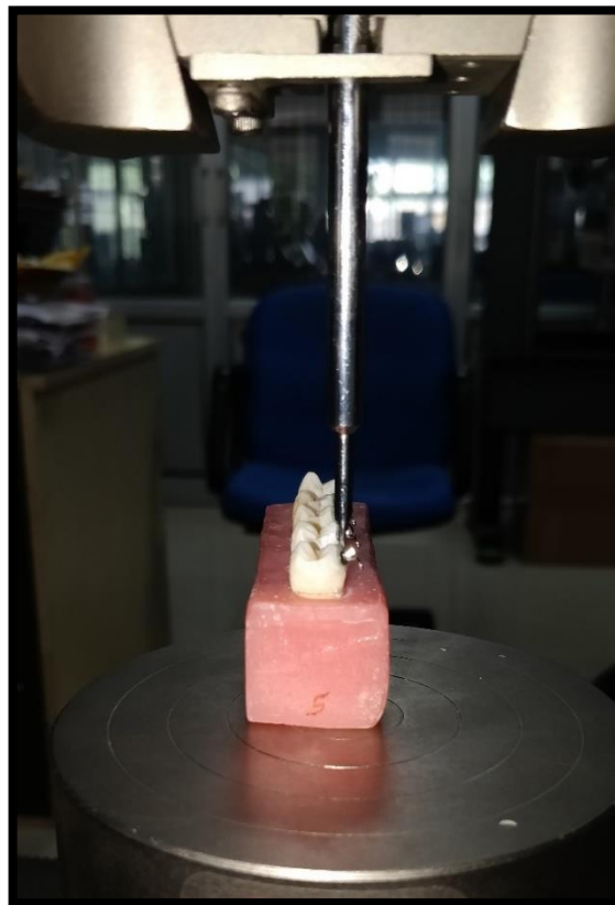
Fig 22. DEBONDING OF BRACKETS BY THE UNIVERSAL TESTING MACHINE
