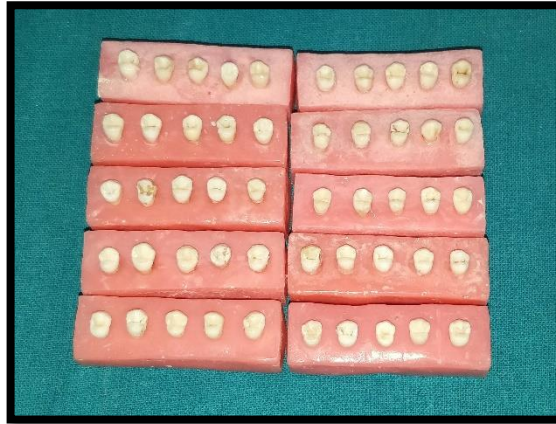
Fig 12. TEETH MOUNTED IN ACRYLIC
