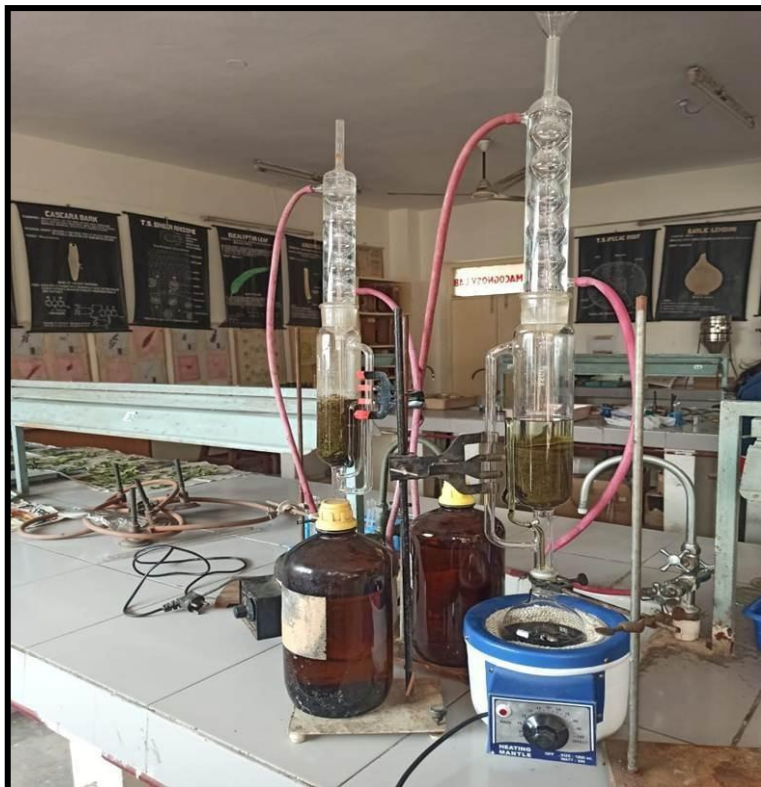
Fig.5: PLANT EXTRACT PREPARATION IN SOXHLET APPARATUS
