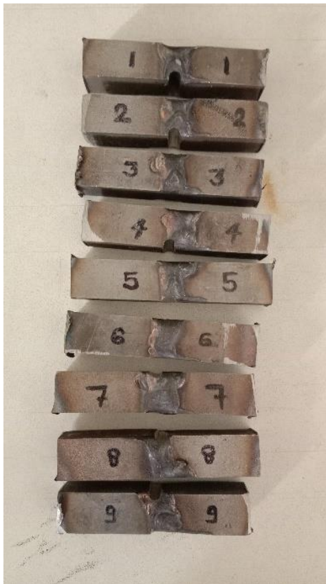
Fig. 4.6 Welded Testing specimen for Impact tests
