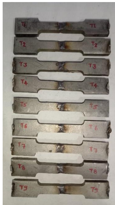
Fig. 4.4 Welded Testing specimen for tensile tests
