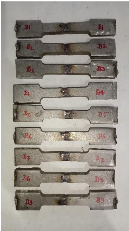
Fig. 4.5 Welded Testing specimen For Bending tests
