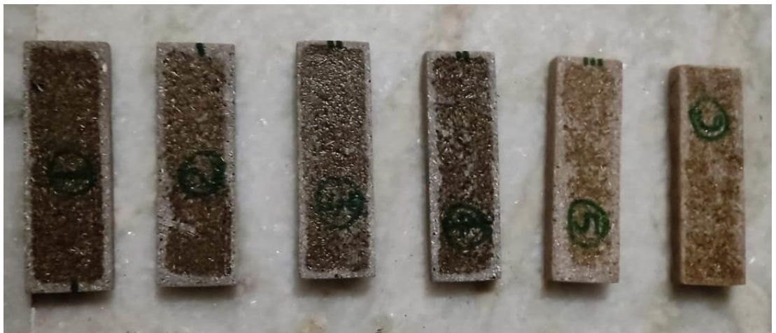
Figure no. :3.9 Prepared specimen for flexural testing
