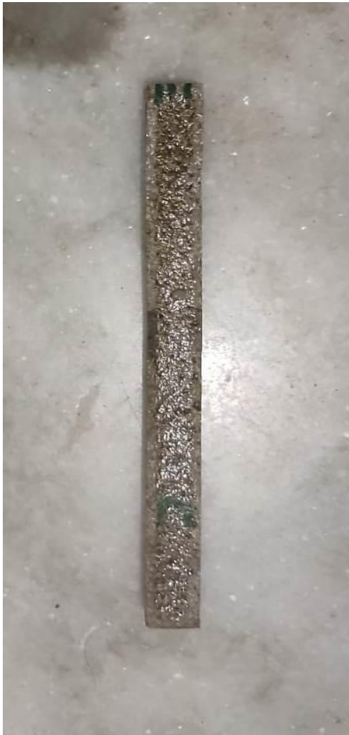
Figure no. :4.8 Before Test Result of C, composite materials, Tensile strength = 8.314 \text{ N/mm}^2 Yield stress = 6.523 \text{ N/mm}^2 Load at peak = 1.3 kN % elongation = 5%
