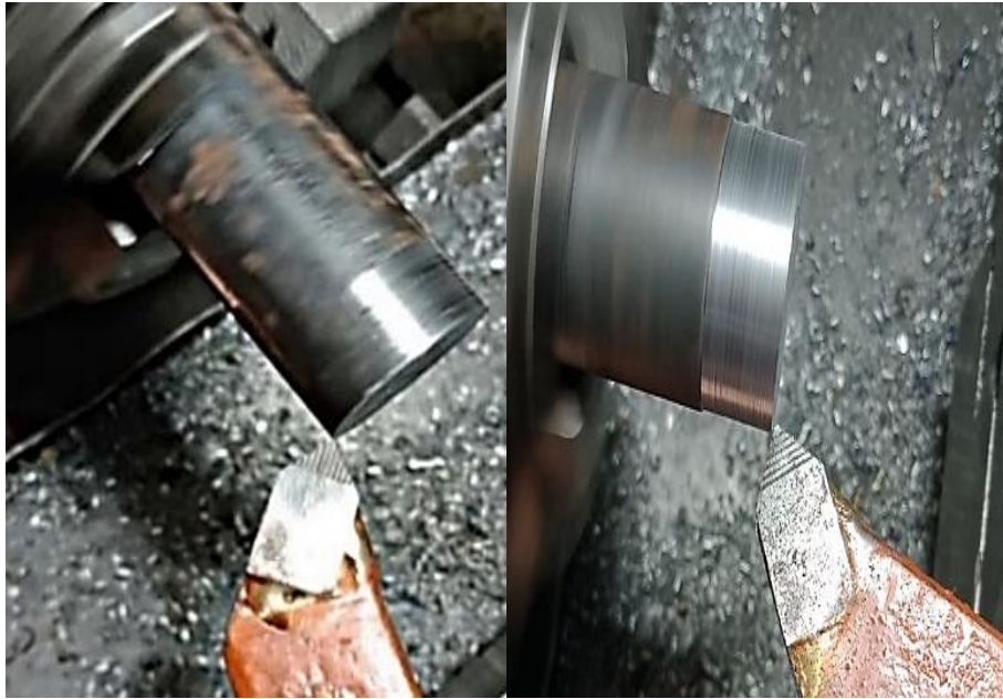
Fig. 3.9 Setup in actual condition for vertical and horizontal textured tools.
