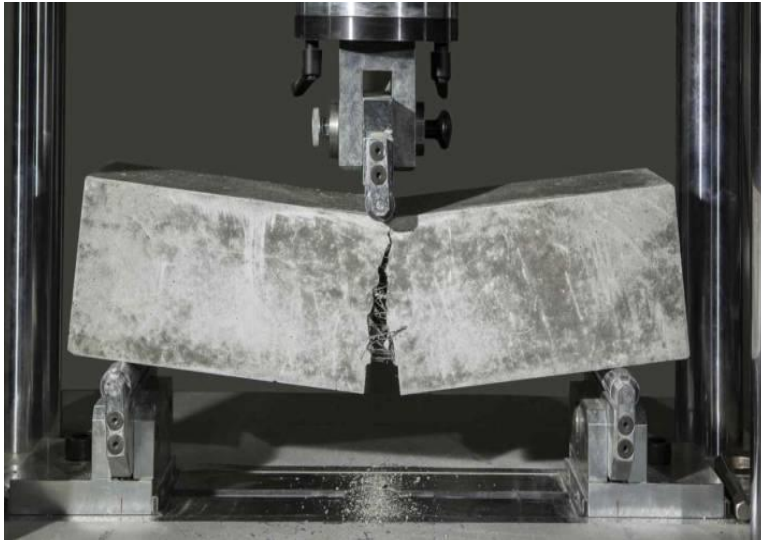
Fig.5. Specimen flexural strength test
