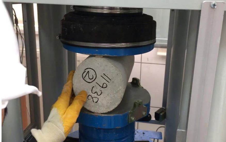
Figure 2. Cylinder under Split tension
