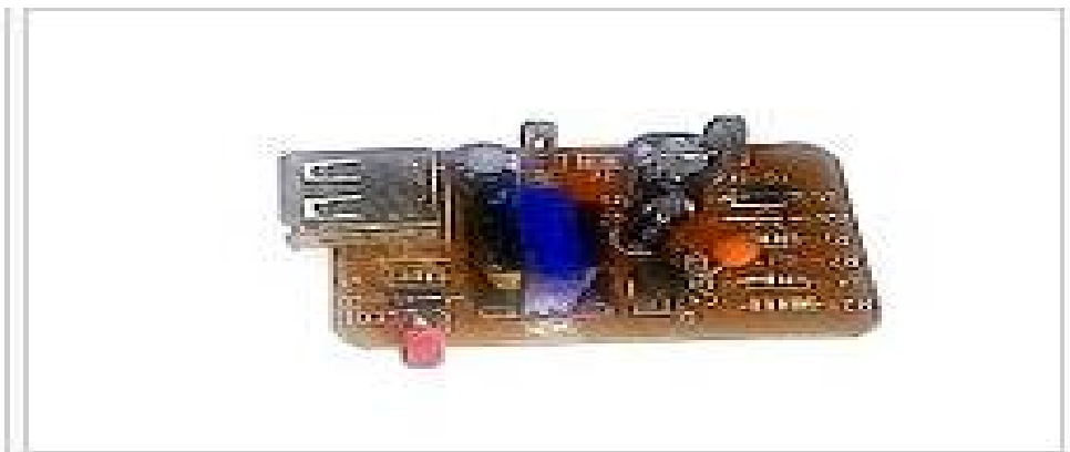
Fig:1.23: Internal circuit of adapter
