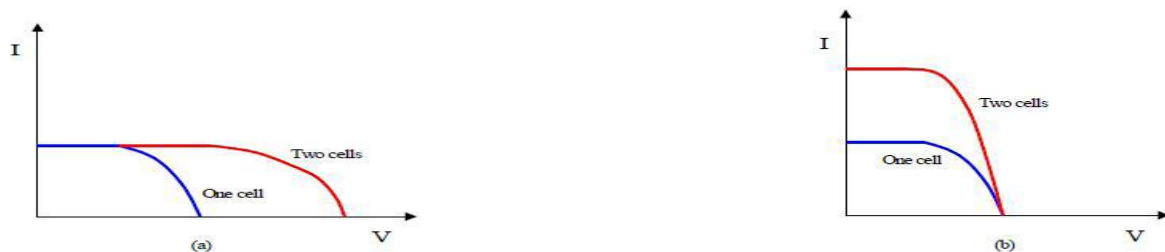
Fig. 2.20 (a): The I - V curve responses with two identical cells connected in series &
