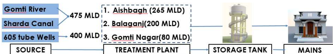
Figure 32 Water Supply System
