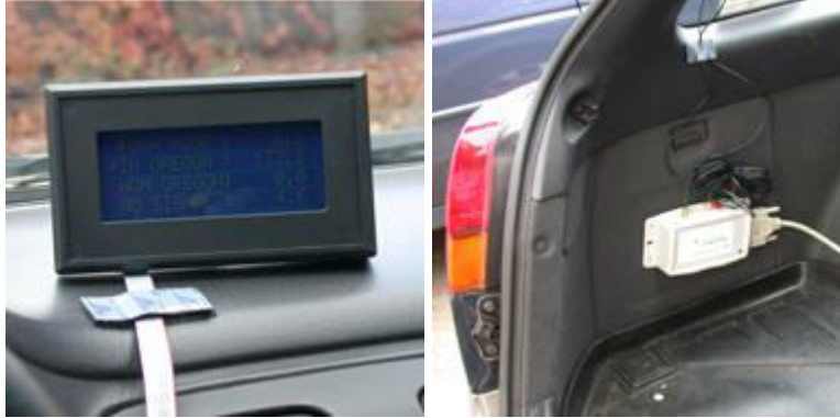
Figure 2.1 On-board mileage-counting equipment in the Oregon Pilot Project [26]
