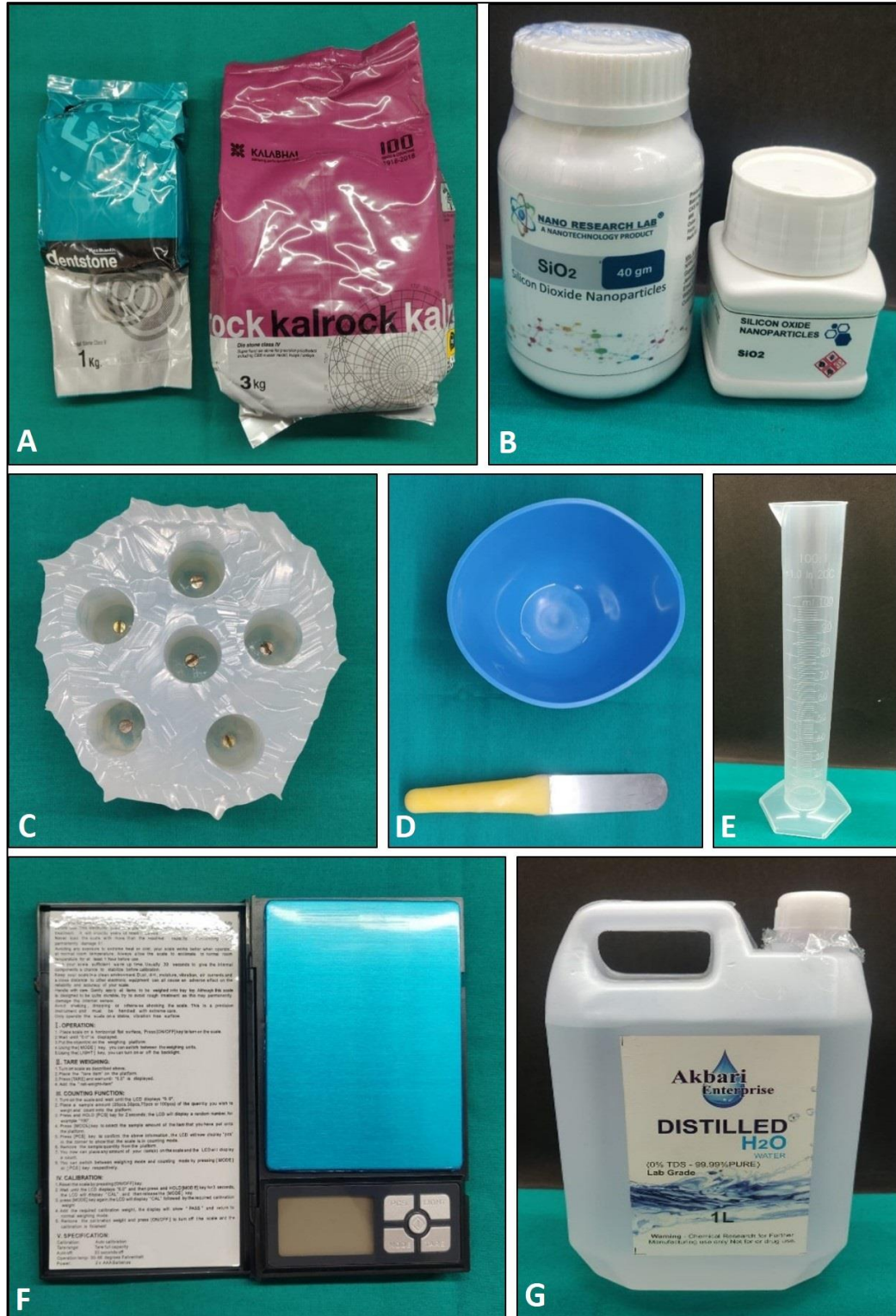
Figure 1: Materials required for preparation of the specimens: A – Dental stone and Die stone; B - Silica nanoparticles; C – Silicone mold; D – Rubber bowl & spatula; E – Measuring cylinder; F – Digital weighing scale; G – Distilled water.
