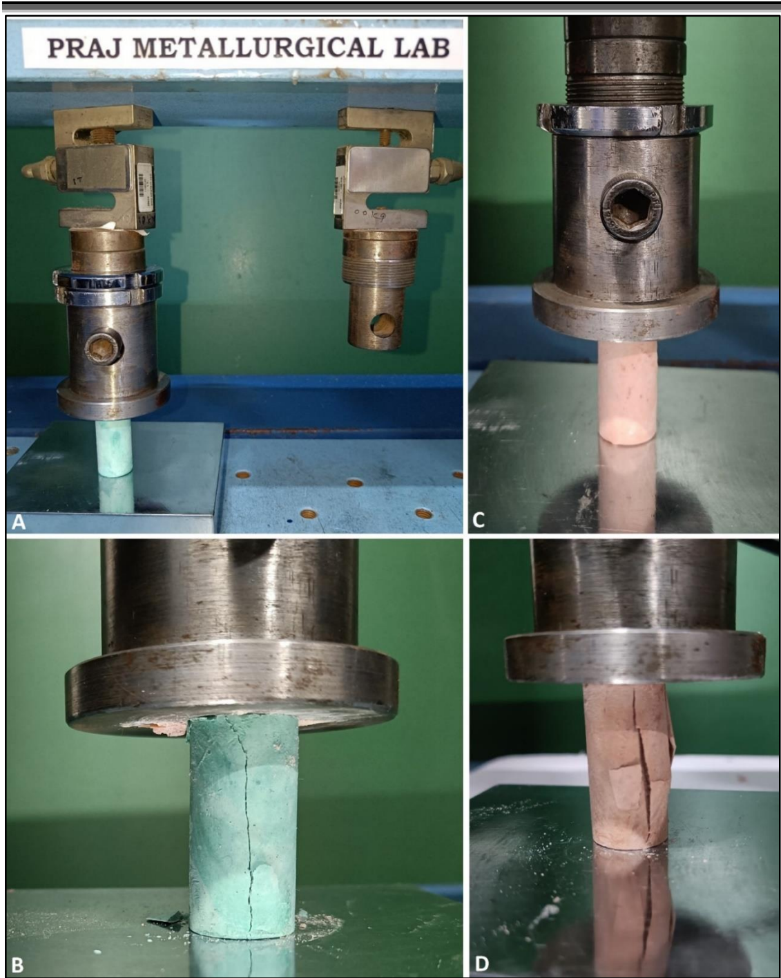
Figure 8: A & B - Dental stone sample during and after compressive strength measurement using Universal testing machine; C & D - Die stone sample during and after compressive strength measurement using Universal testing machine
