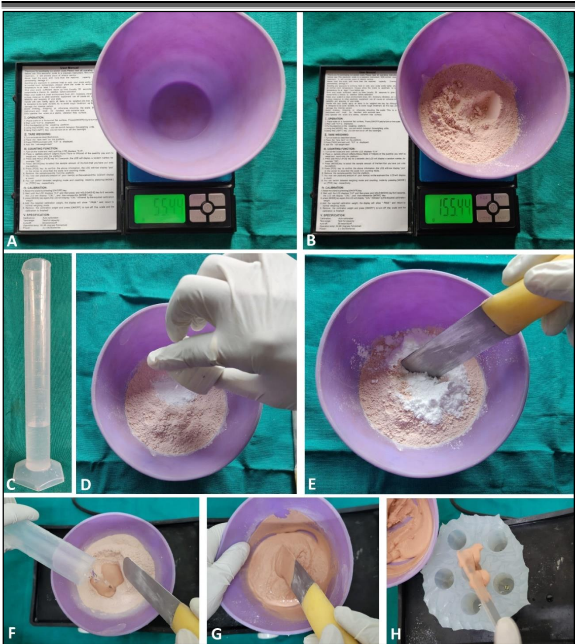
Figure 4: A & B – Measuring 100gm of die stone powder; C – Measuring cylinder to measure 23 ml of distilled water; D & E - Mixing silica nanoparticles to die stone powder to obtain a uniform mix; E – Distilled water being added to the powder; G & H- The stone being mechanically spatulated and poured into the silicone mold under vibration.
