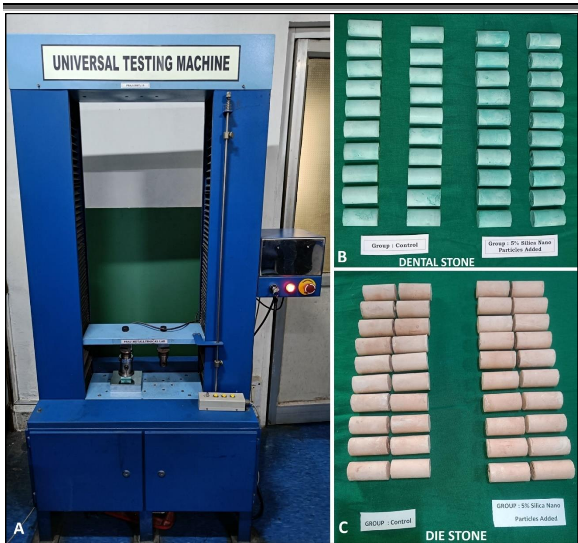
Figure 6: A – Universal testing machine (UTM) for testing Diametral tensile strength and Compressive strength of dental stone and die stone; B – Dental stone (Control and test groups); C – Die stone (Control and test groups)
