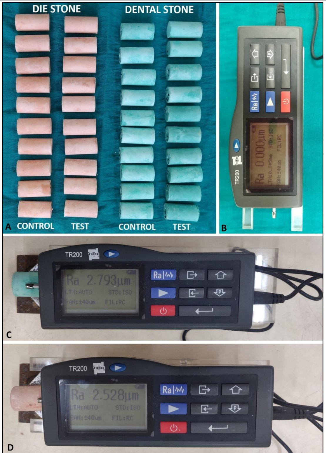
Figure 5: A – Die stone and dental stone samples (Control and test groups); B – Calibrating TR200 to zero; C – Measuring surface roughness of Dental stone using TR200; D - Measuring surface roughness of Die stone using TR200.
