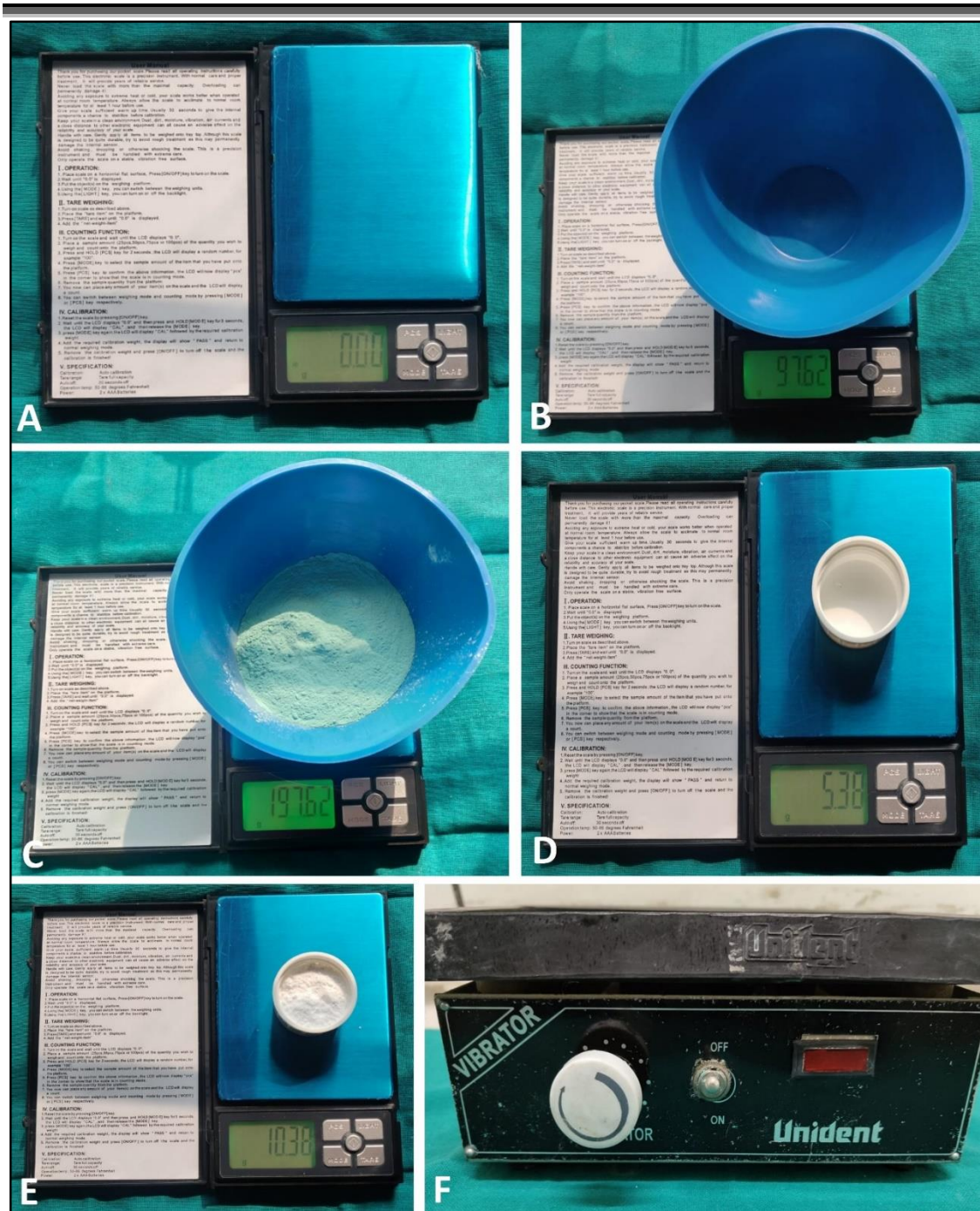
Figure 2: A – Calibrating digital weighing scale to zero; B & C – Measuring 100gm of dental stone powder; D & E - Measuring 5gm of silica nanoparticles; F - Vibrator
