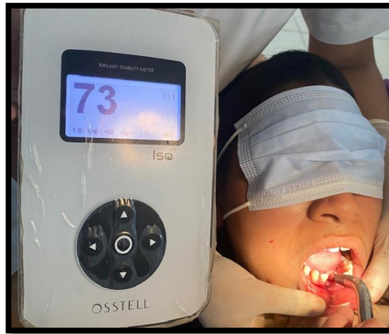
Figure 12: Primary stability measurement using Osstell ISQ device
